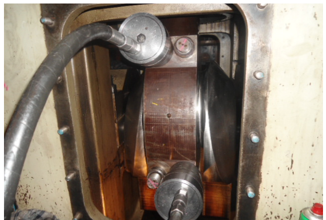
Connecting rod bolt/nut tightening
