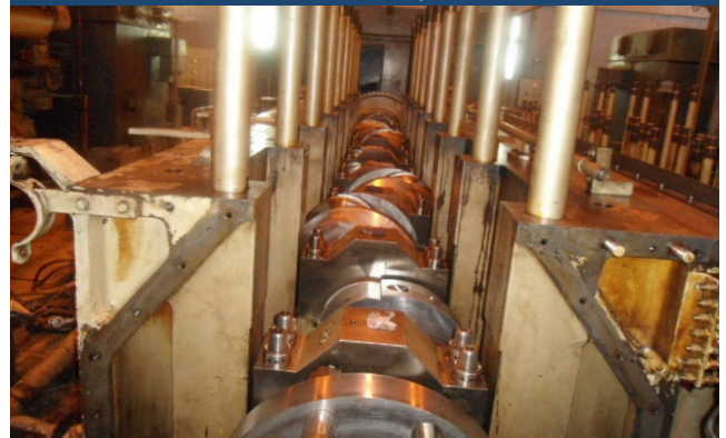
New crankshaft fitted on bedplate
