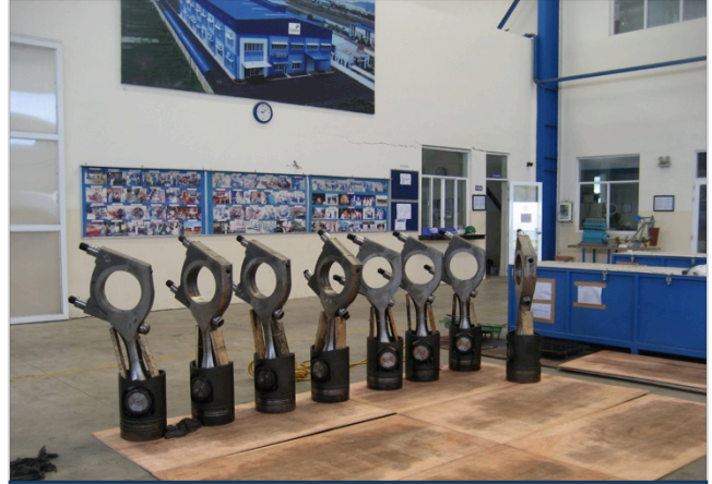
Piston assemblies in workshop for overhaul
