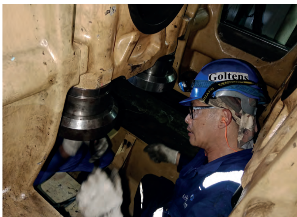
Technician tightening main bearing cap to check the pocket bore alignment
