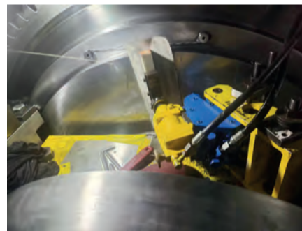
Thrust collar surface honing after machining
