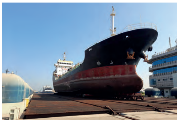
Tanker being raised by DMC synchrolift for service
