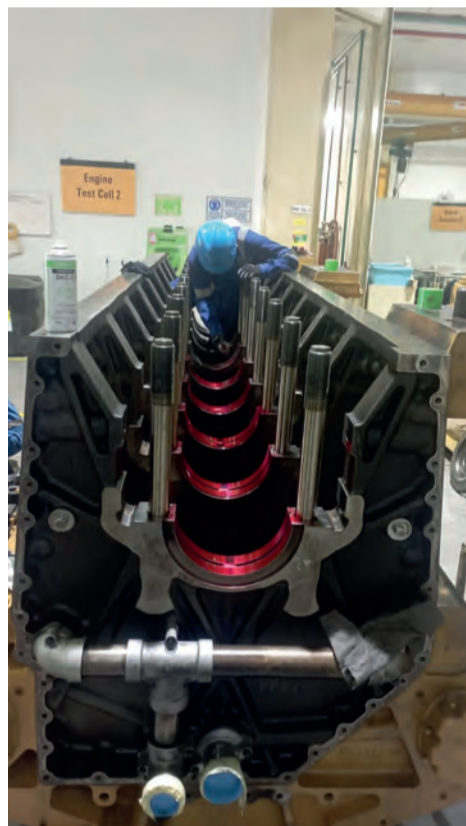
Crack test on bearing pockets
