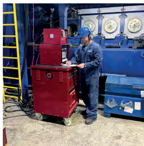
Goltens' specialist monitoring heating and cooling process on crankpin
