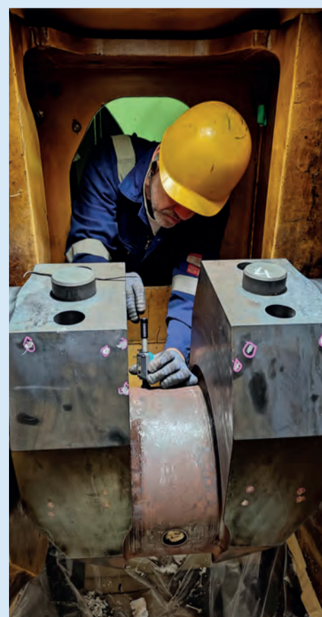
Hardness checks on crankpin journal after annealing and cooling
