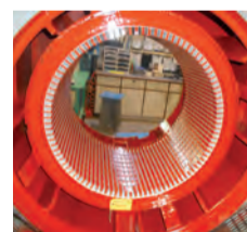
Stator after rewinding
