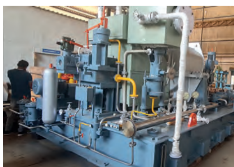
Fully reconditioned steam turbine ready for dispatch
