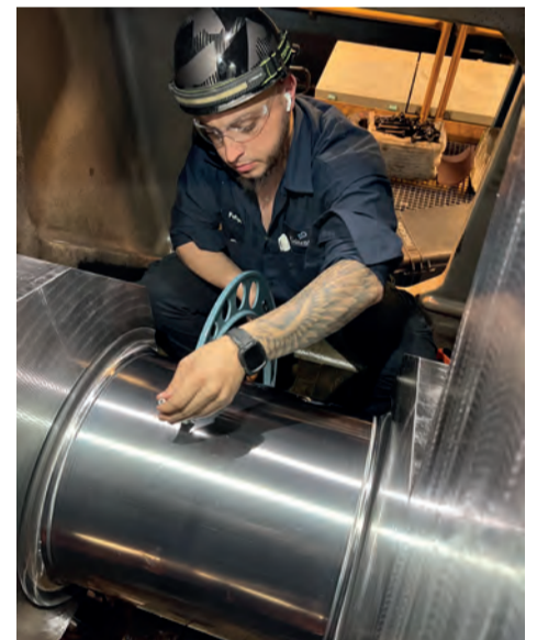
Calibration check on one of the engine's crankpin journals
