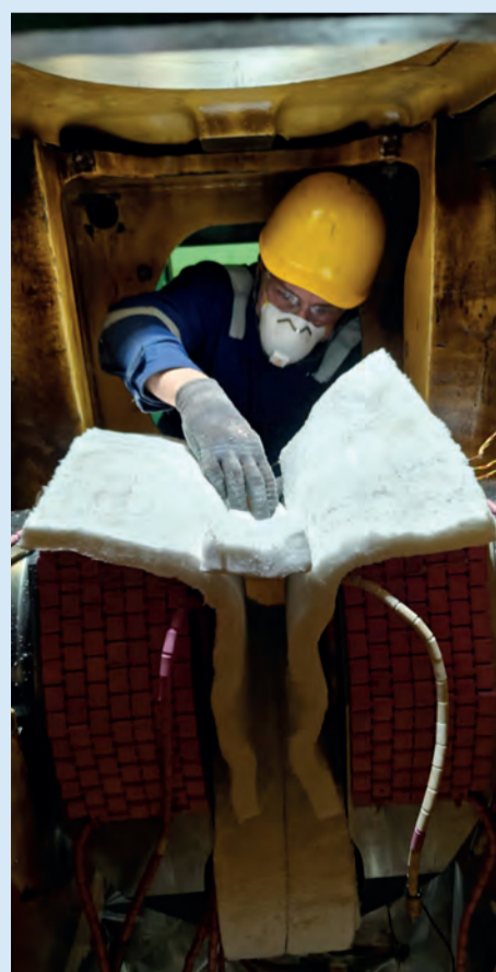
Installation of ceramic tiles on one of the crankpins in preparation for annealing
