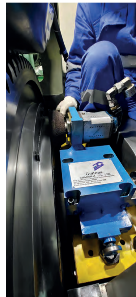
Customized In-Place Machining tools developed by Goltens installed for repair
