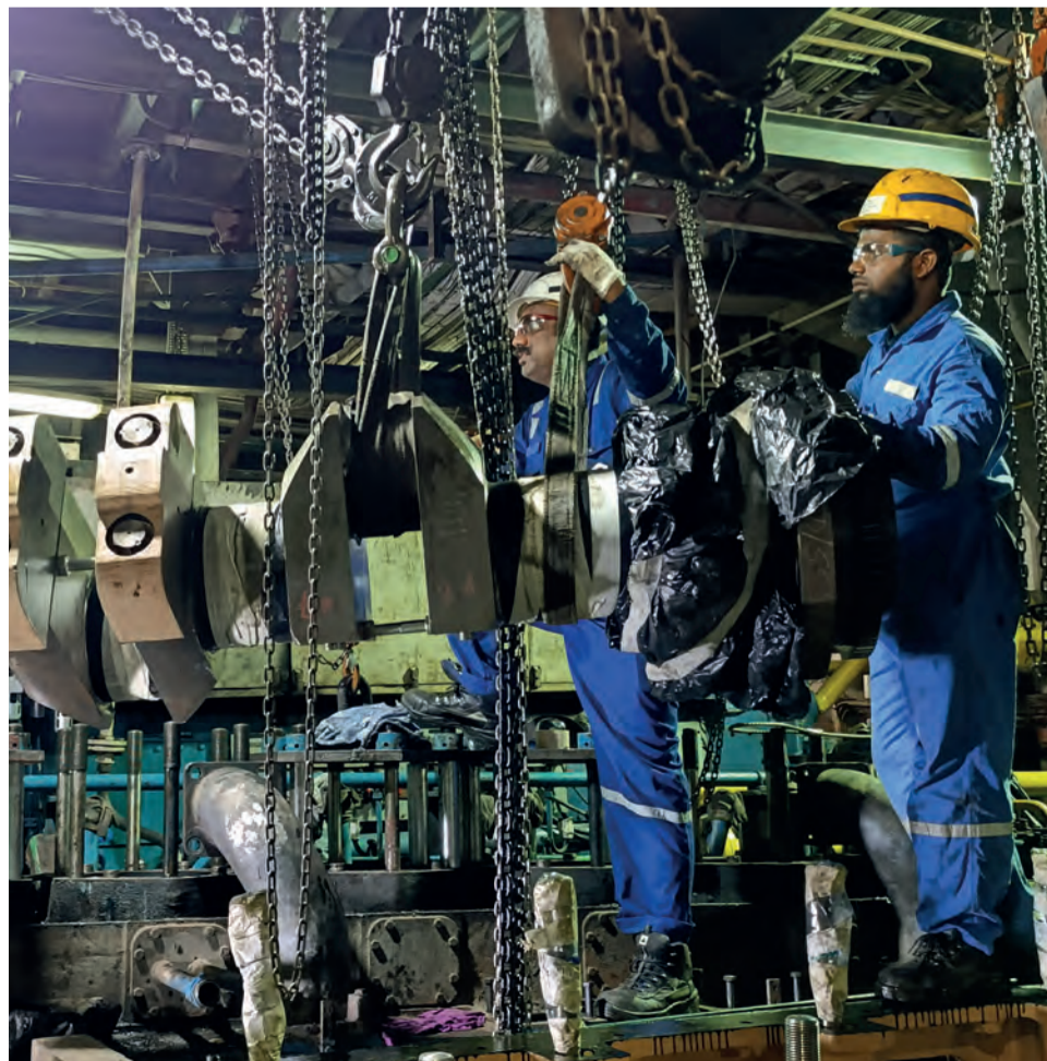
Goltens' specialists rigging crankshaft out of the block in engine room
