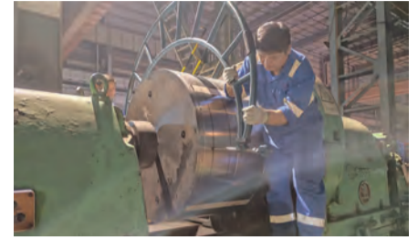
Measurement of new stern tube bearing
