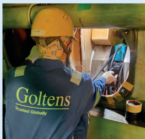
Machining of one of the successfully annealed crankpins
