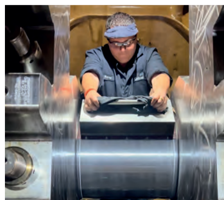
Technician using custom-manufactured mandrel to remove ridge wear
