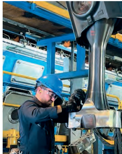
Rigging of one of the piston assemblies to the floor for inspection
