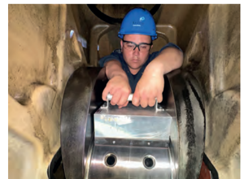
Lapping dummy employed to remove ridge wear found on Engine No.9 to reduce 'point load' risk on rebuild
