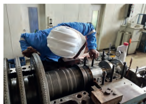
Performance of run-out checks on the turbine rotor
