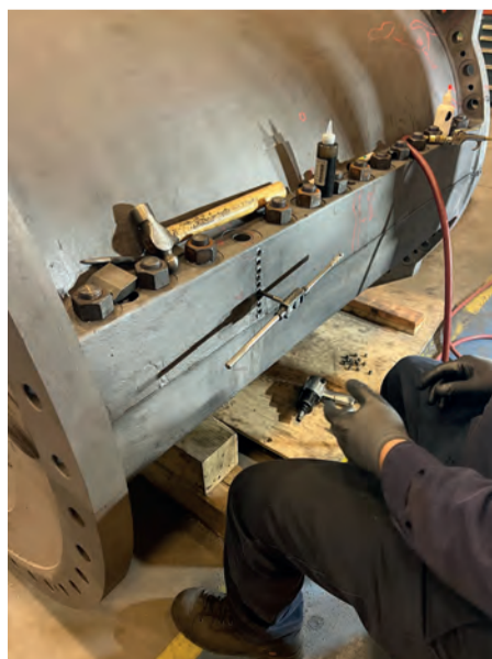
Tapping holes for second set of stitching pins
