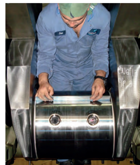
Checking running surface for ridge wear with straight edge
